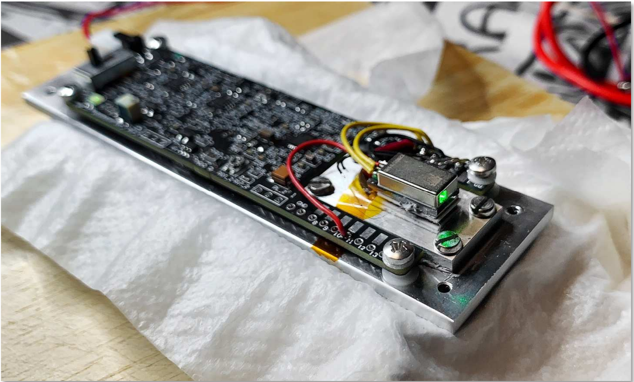
Above & Lower Left – Laser Operating on Cold block – 4 October 2022
