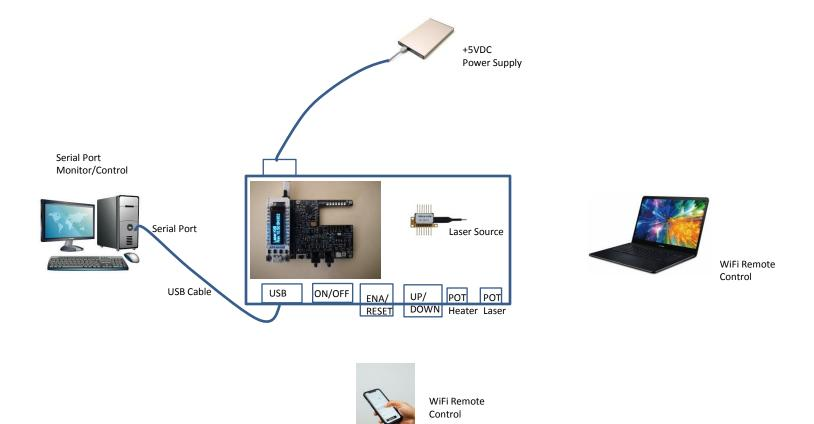
Laser Drive Board Connection Diagram
